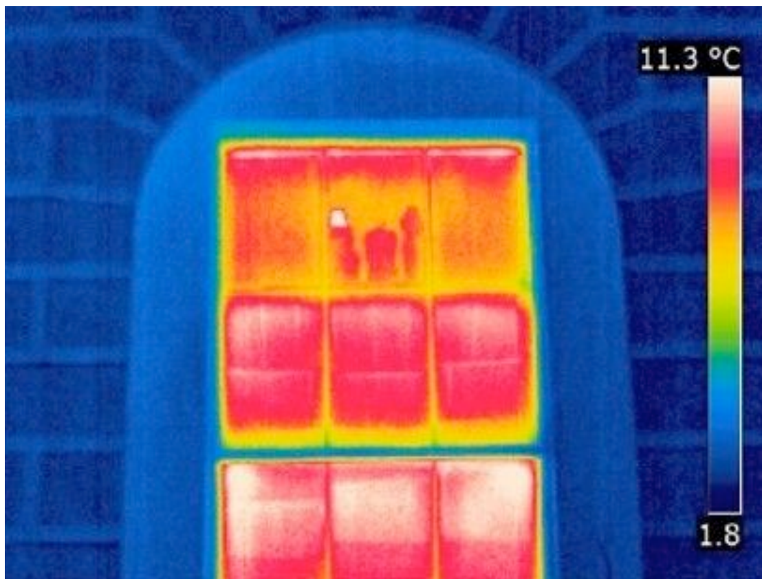
Figure 1 Thermal image showing dramatic heat loss through single glazing
