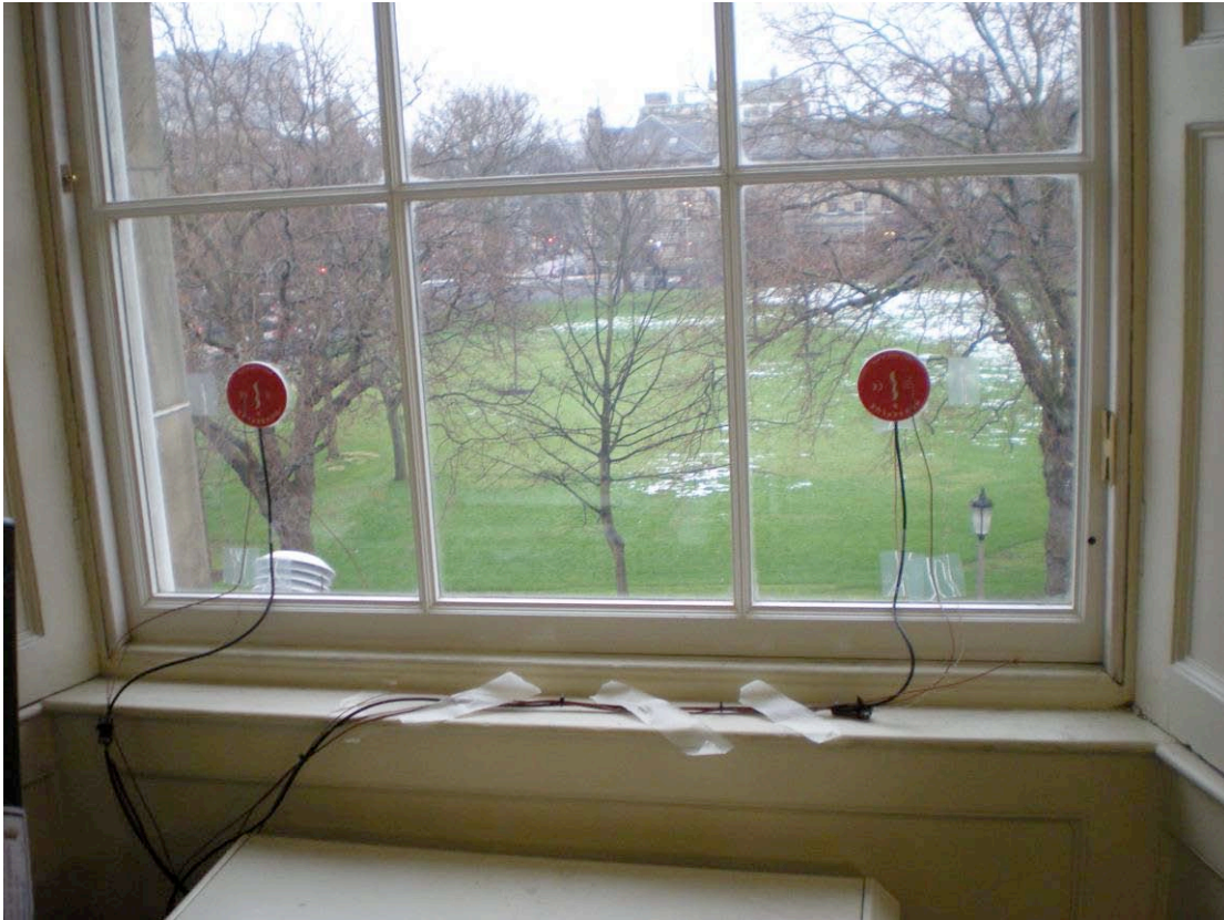
Figure 1: Typical test arrangement on glazing in Georgian sash
